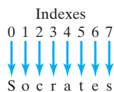
Figure 7.6: The string “Socrates” has eight characters, indexed from 0 to 7. This is an example of zero indexing .
