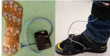
**Figure 1.** (Left) Flexible PCB with embedded sensors and the control pack containing the WiFi-enabled microcontroller and the 3.3-VLi-ion battery; (Right) a user showing the padded SmartInsole in a sandal while strapping the control pack around the leg.
