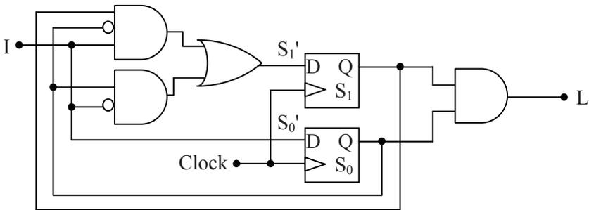
**Figure 11-26** Final Circuit to Identify the Bit Pattern "101"
