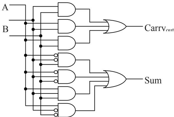
**Figure 8-8** Logic Circuit for a Full Adder
