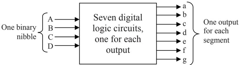
**Figure 8-12** Block Diagram of a Seven-Segment Display Driver
