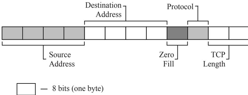
**Figure 14-6** Layout of a TCP Pseudo Header
