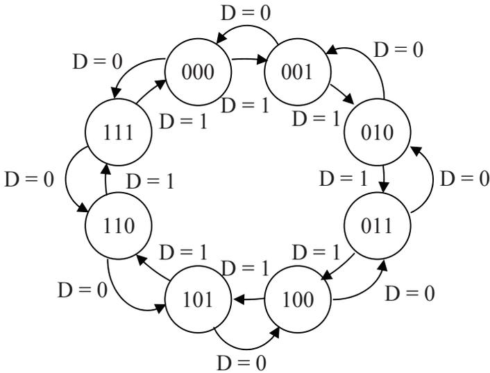
**Figure 11-7** State Diagram for a 3-Bit Up-Down Binary Counter
