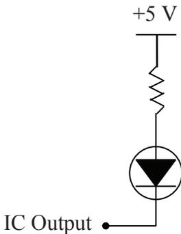
**Figure 8-36** LED Circuit
