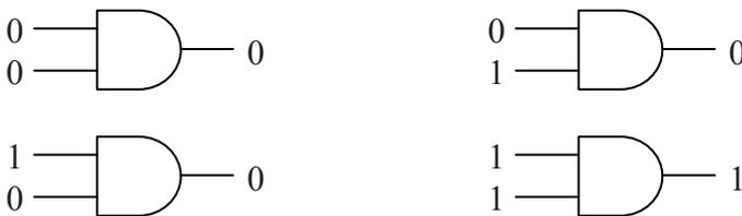
**Figure 4-4** Operation of a Two-Input AND Gate
