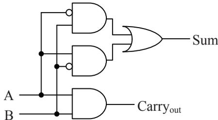
**Figure 8-4** Logic Circuit for a Half Adder
