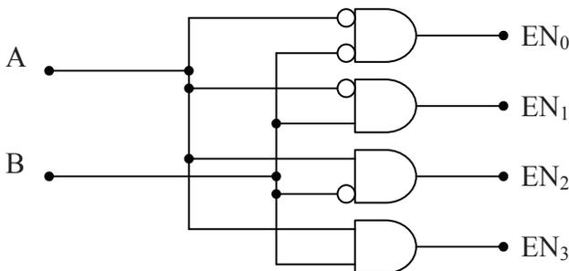
**Figure 8-22** Digital Circuit for a 1-of-4 Decoder
