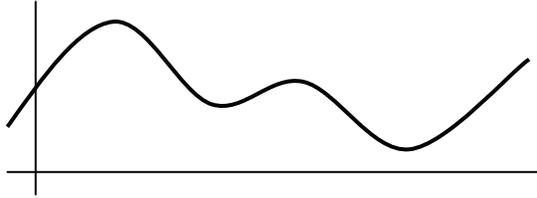
**Figure 1-2** Continuous Analog Signal with Infinite Resolution
