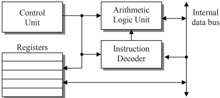
**Figure 15-5** Generic Block Diagram of a Typical CPU
