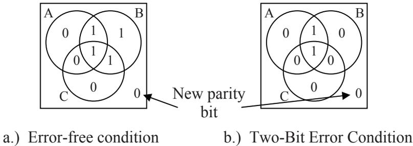
**Figure 9-15** Using Parity to Check for Double-Bit Errors
