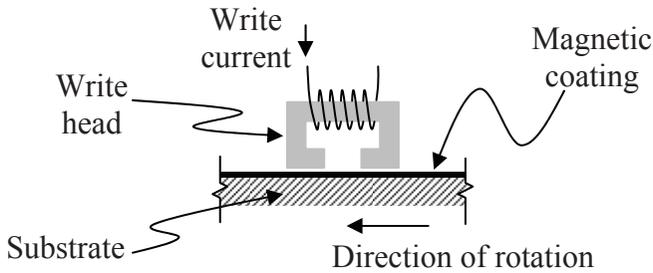
**Figure 13-2** Configuration of a Hard Drive Write Head
