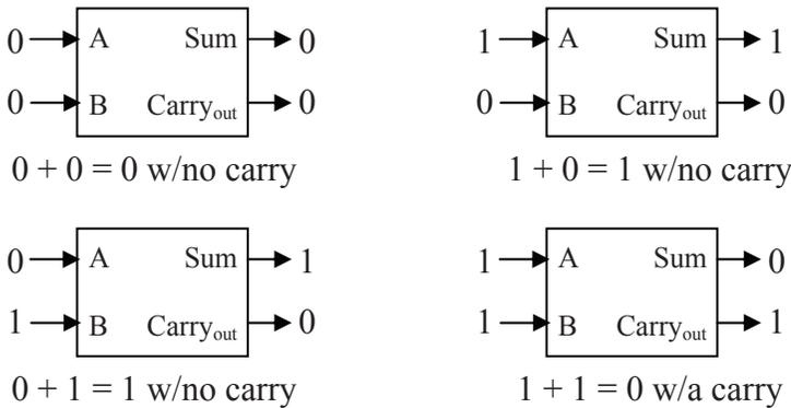
**Figure 8-3** Four Possible States of a Half Adder
