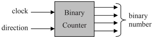
**Figure 11-6** Block Diagram of an Up-Down Binary Counter
