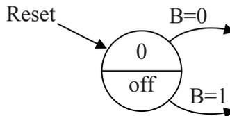
**Figure 11-11** Transitions from State 0 of Push Button Circuit
