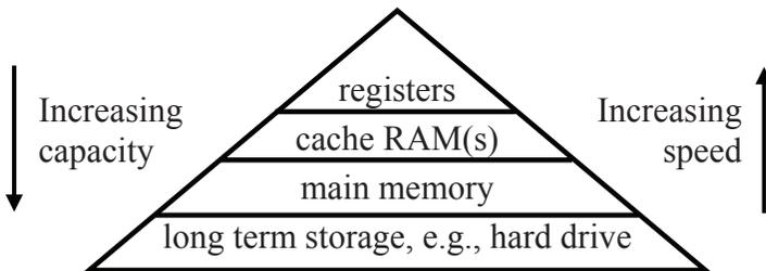
**Figure 13-1** Block Diagram of a Standard Memory Hierarchy
