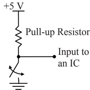
**Figure 8-37** Switch Circuit
