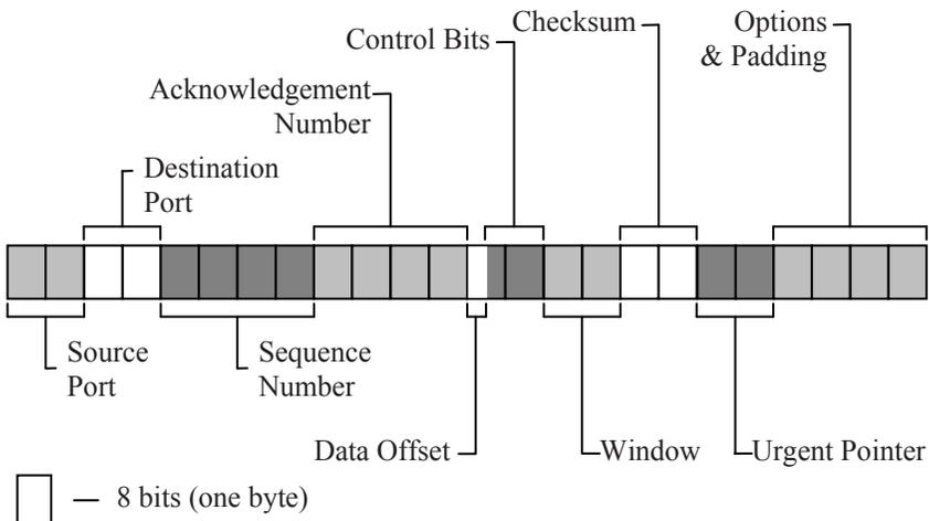
**Figure 14-4** Layout of a TCP Packet Header
