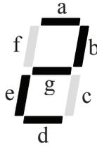
**Figure 8-11** A Seven-Segment Display Displaying a Decimal '2'
