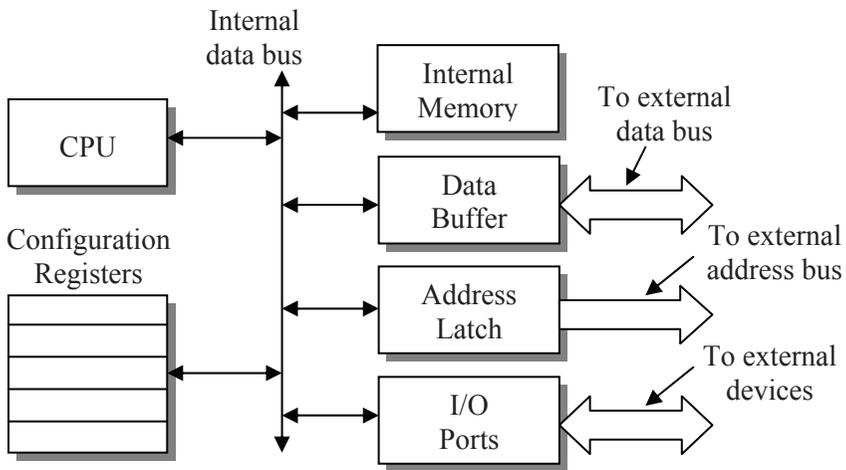
**Figure 15-4** Generic Block Diagram of Processor Internals
