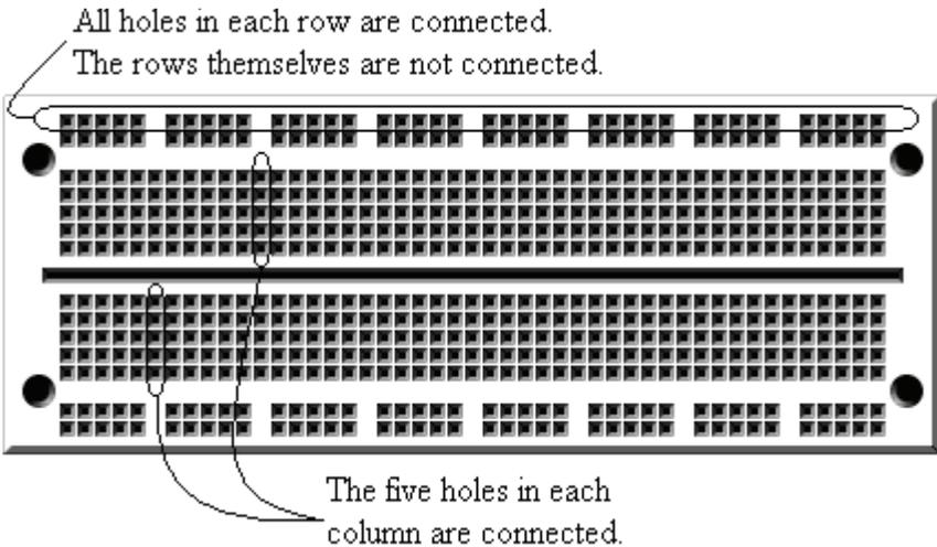
**Figure 8-33** Generic Protoboard Internal Connections
