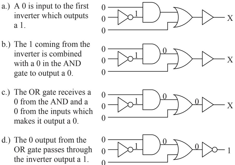
**Figure 4-23** Process of Passing Inputs Through Combinational Logic
