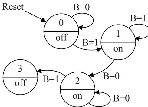
**Figure 11-16** Transitions from State 2 of Push Button Circuit
