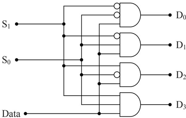
**Figure 8-27** Logic Circuit for a 1-Line-to-4-Line Demultiplexer
