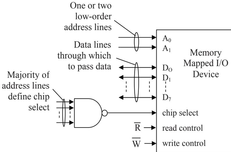
**Figure 15-9** Sample Memory Mapped Device Circuit
