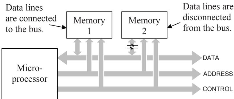
**Figure 12-4** Two Memory Devices Sharing a Bus
