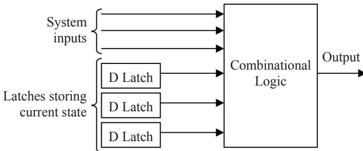
**Figure 11-1** Adding Memory to a Digital Logic Circuit
