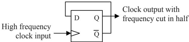
**Figure 10-14** Divide-By-Two Circuit
