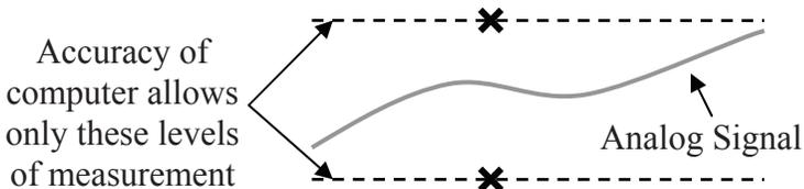
**Figure 1-6** Poor Resolution Resulting in an Inaccurate Measurement
