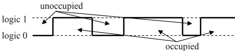
**Figure 9-4** Possible Output from a Motion Detector
