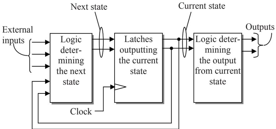
**Figure 11-9** Block Diagram of a State Machine
