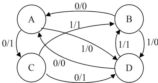
**Figure 11-28** Sample State Diagram of a Mealy Machine
