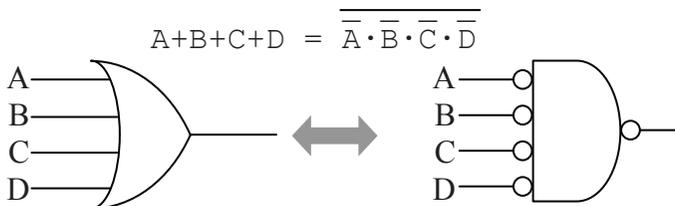
**Figure 6-12** OR-to-NAND Equivalency Expanded to Four Inputs
