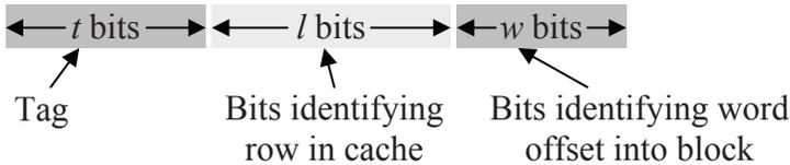
**Figure 13-20** Direct Mapping Partitioning of Memory Address
