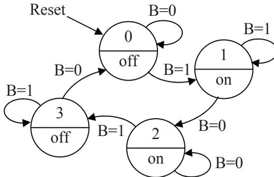
**Figure 11-17** Final State Diagram for Push Button Circuit
