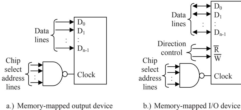
**Figure 12-10** Some Types of Memory Mapped I/O Configurations
