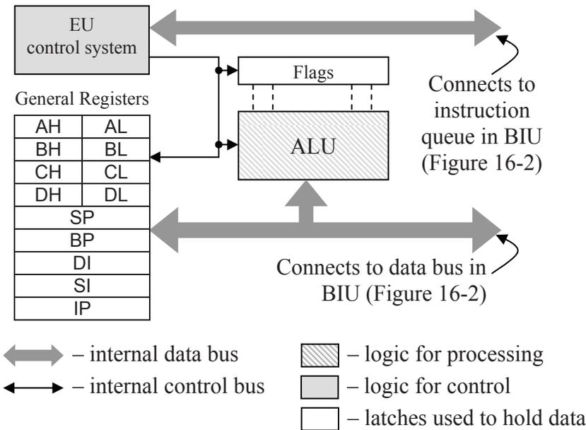
**Figure 16-1** Block Diagram of 80x86 Execution Unit (EU)
