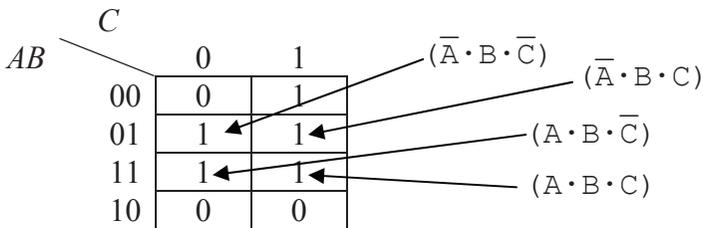
**Figure 7-6** Karnaugh Map with Four Adjacent Cells Containing '1'
