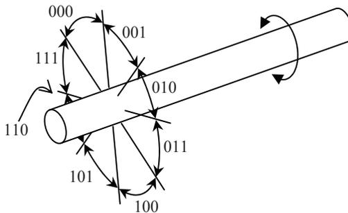
**Figure 2-10** Eight Binary Values Identifying Rotating Shaft Position
