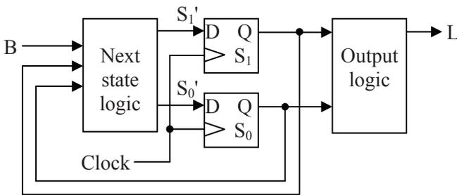
**Figure 11-18** Block Diagram for Push Button Circuit
