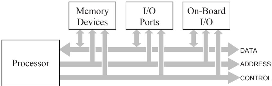
**Figure 15-3** Generic Block Diagram of a Processor System
