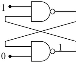
a.) A zero to the free input of the bottom NAND gate forces a one to its output
