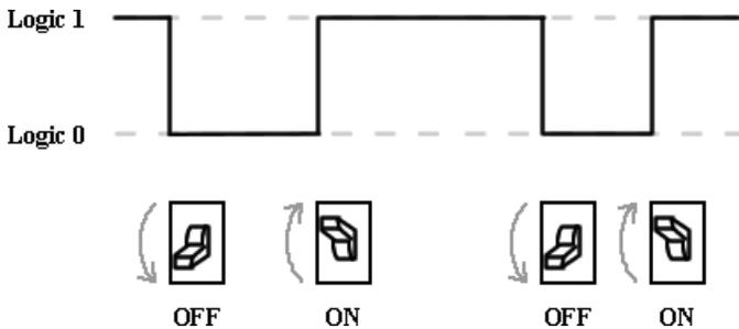
**Figure 1-8** Representation of a Single Binary Signal
