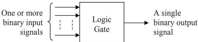
**Figure 4-1** Basic Format of a Logic Gate
