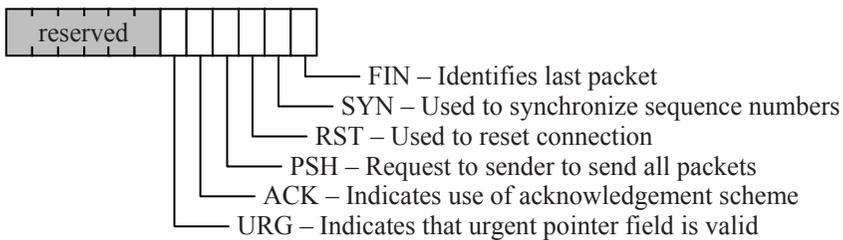
**Figure 14-5** Position and Purpose of TCP Control Flags
