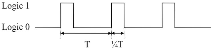
**Figure 1-16** Periodic Pulse Train with 25% Duty Cycle
