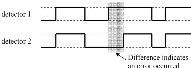
**Figure 9-5** A Difference in Output Indicates an Error
