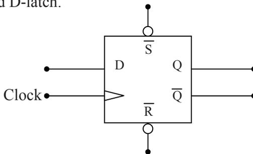
Figure 10-11 Block Diagram of the D Latch
