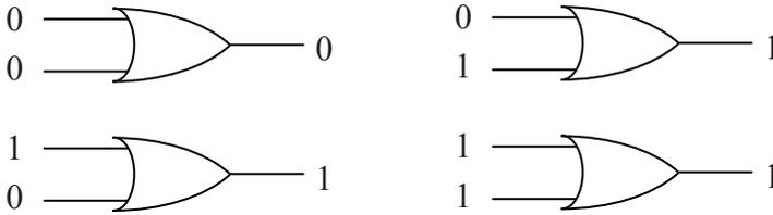
**Figure 4-5** Operation of a Two-Input OR Gate
