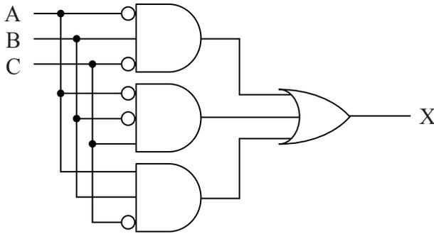
**Figure 6-13** Sample SOP Circuit
