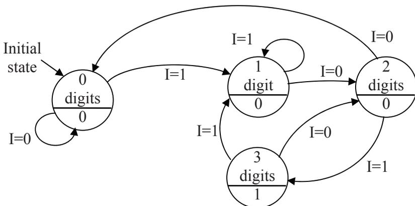
**Figure 11-23** State Diagram for Identifying the Bit Pattern "101"
