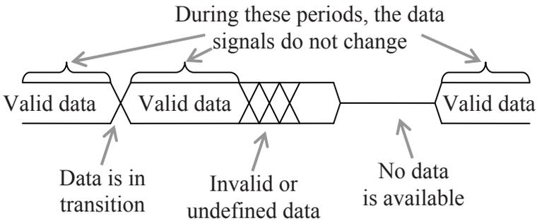
**Figure 1-10** Alternate Representation of Multiple Digital Signals
