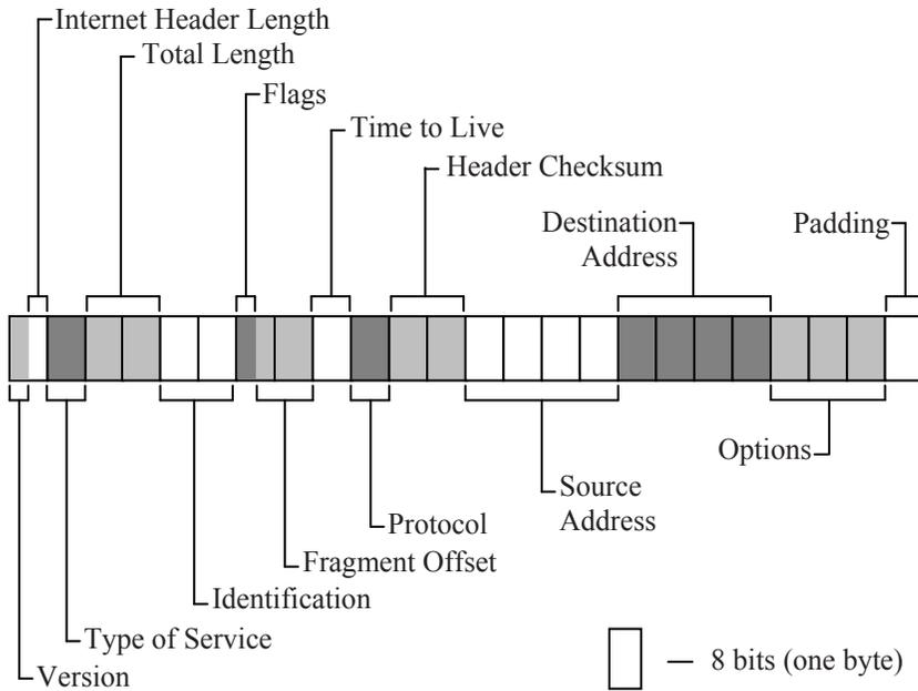
**Figure 14-3** Layout of an IP Packet Header
