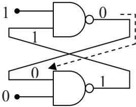
c.) A zero from the top NAND returns to the lower input of the bottom NAND
