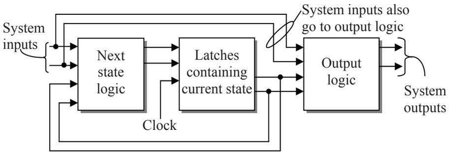
**Figure 11-27** Basic Configuration of a Mealy Machine
