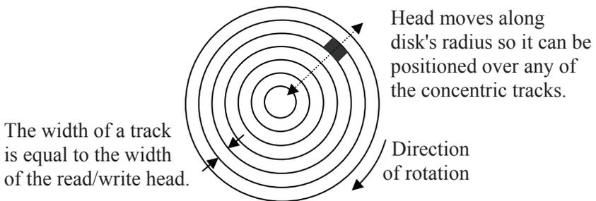
**Figure 13-8** Relation between Read/Write Head and Tracks
