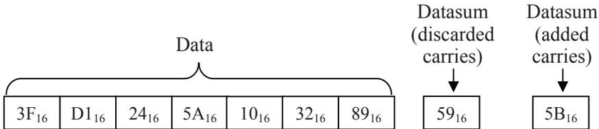
**Figure 9-7** Sample Block of Data with Accompanying Datasums
