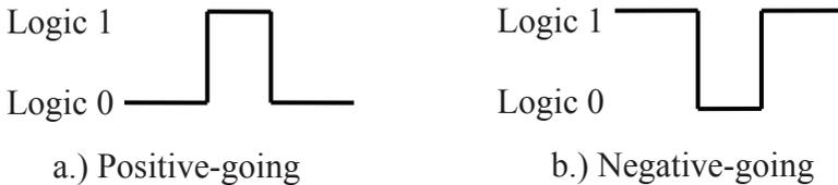
**Figure 1-12** Pulse Waveforms
