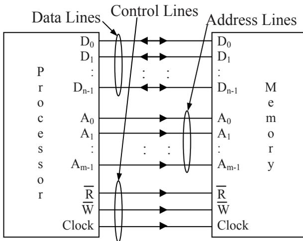
**Figure 12-3** Basic Processor to Memory Device Interface
