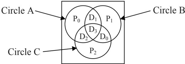
**Figure 9-12** Venn Diagram Representation of Hamming Code
