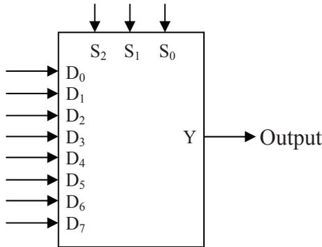
**Figure 8-25** Block Diagram of an Eight Channel Multiplexer
