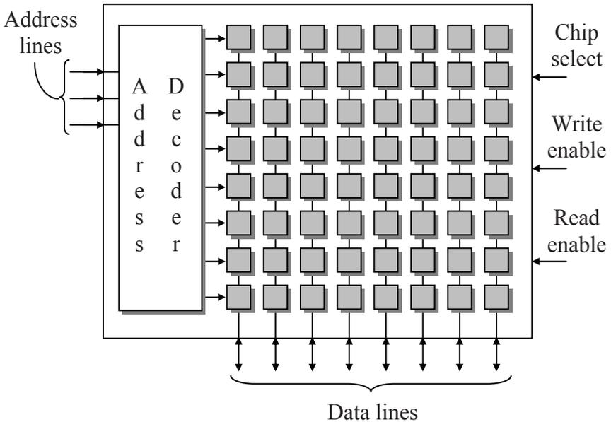
**Figure 12-2** Basic Organization of a Memory Device
