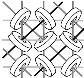
**Figure 12-1** Diagram of a Section of Core Memory
