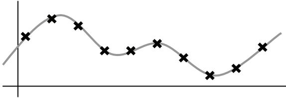
**Figure 1-4** Samples Taken of an Analog Signal
