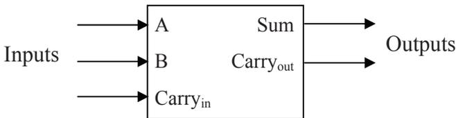
**Figure 8-6** Block Diagram of a Full Adder
