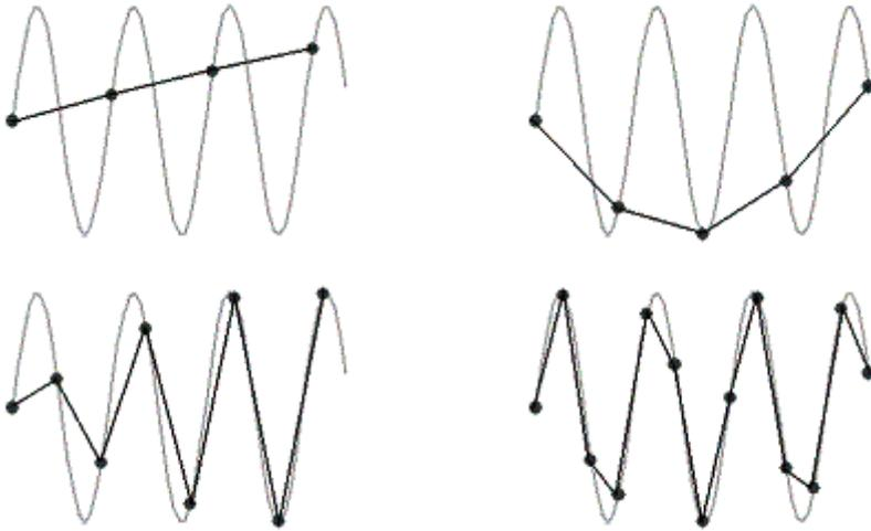
**Figure 2-9** Aliasing Effects Due to Slow Sampling Rate
