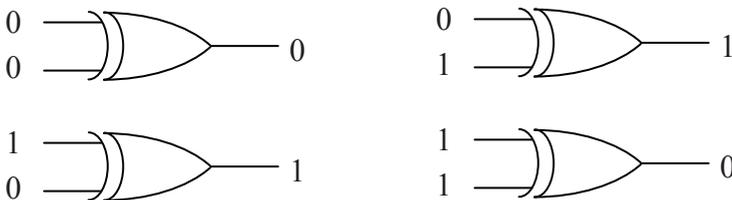
**Figure 4-6** Operation of a Two-Input XOR Gate
