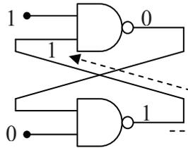
b.) That one passes to the top NAND which in turn outputs a zero
