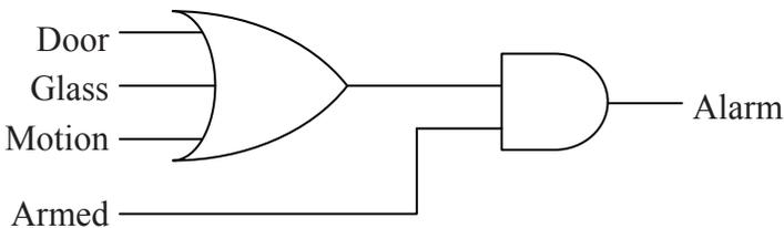
**Figure 4-18** Combinational Logic for a Simple Security System
