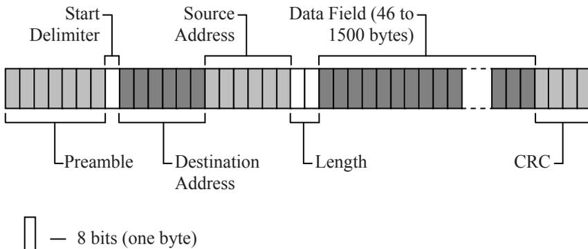
**Figure 14-2** Layout of an IEEE 802.3 Ethernet Frame
