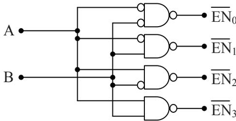
**Figure 8-23** Digital Circuit for an Active-Low 1-of-4 Decoder
