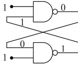
d.) The second zero at the bottom NAND holds its output even if the free input returns to 1
