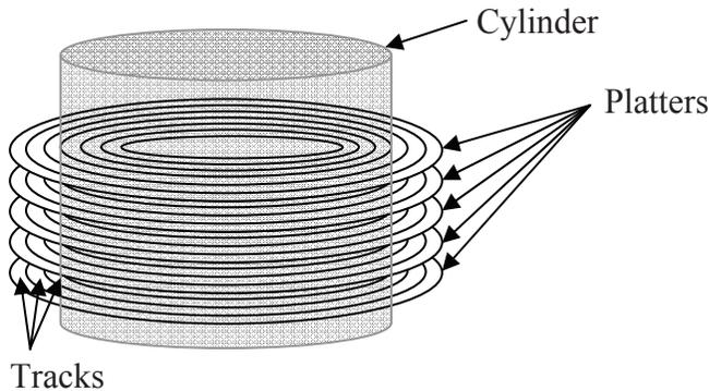
**Figure 13-10** Illustration of a Hard Drive Cylinder
