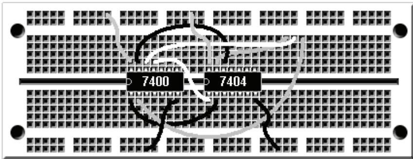
**Figure 8-34** Sample Circuit Wired on a Protoboard
