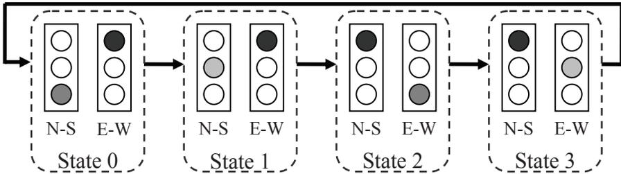
**Figure 11-2** States of a Traffic Signal System
