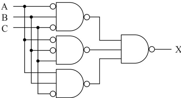
**Figure 6-15** Sample SOP Circuit Implemented With NAND Gates
