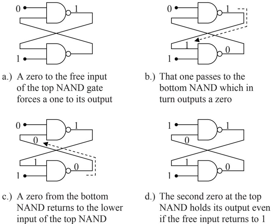
**Figure 10-7** Operation of a Simple Memory Cell
