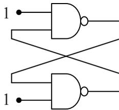
**Figure 10-5** Primitive Feedback Circuit Redrawn with NAND Gates
