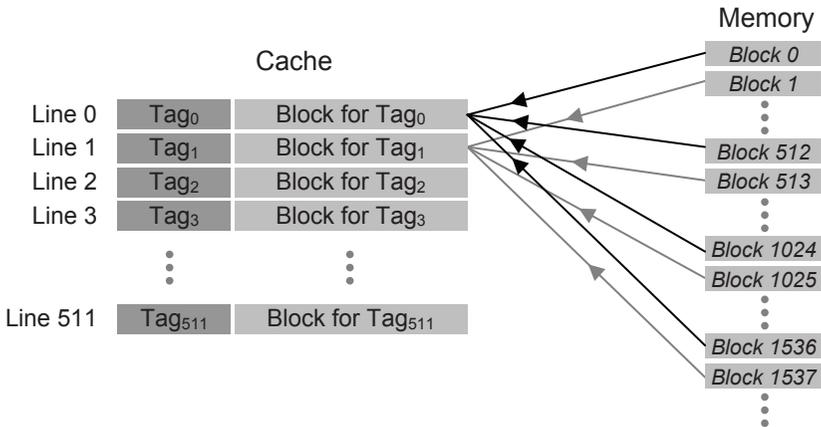
**Figure 13-19** Direct Mapping of Main Memory to Cache
