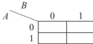
**Figure 7-1** 2-by-2 Karnaugh Map Used with Two Inputs
