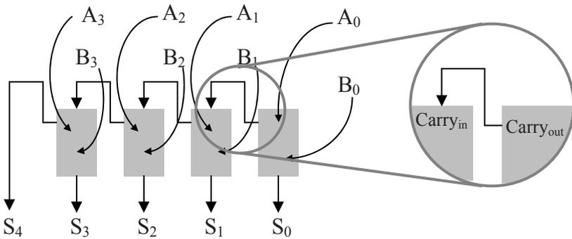
**Figure 8-5** Block Diagram of a Multi-bit Adder
