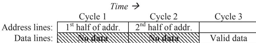
**Figure 12-11** Basic Addressing Process for a DRAM
