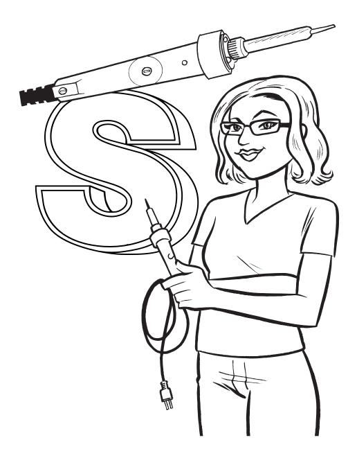
A **soldering iron** is like a hot glue gun for electronics, except instead of glue, it melts metals like silver, tin and lead. Using metals to build electronic devices is important because metal conducts electricity. When the metal cools and hardens, it fixes the components in place, connects them electrically, and keeps them from moving around.
