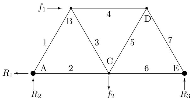
Figure 9.1: An equilateral truss. Joints or nodes are labeled alphabetically,  $A, B, \dots$  and Members (edges) are labeled numerically:  $1, 2, \dots$ . The forces  $f_1$  and  $f_2$  are applied loads and  $R_1, R_2$  and  $R_3$  are reaction forces applied by the supports.
