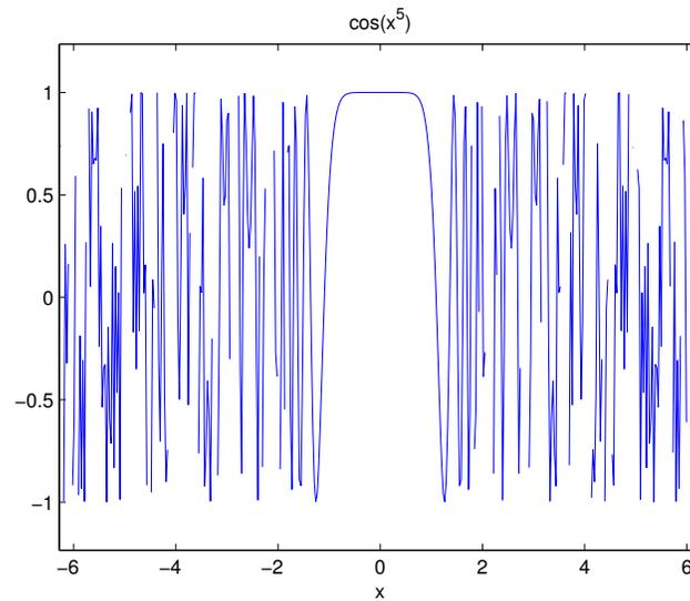
Figure 7.1: Graph of  $\cos(x^5)$  produced by the `ezplot` command. It is wrong because  $\cos u$  should oscillate smoothly between  $-1$  and  $1$ . The problem with the plot is that  $\cos(x^5)$  oscillates extremely rapidly, and the plot did not consider enough points.
