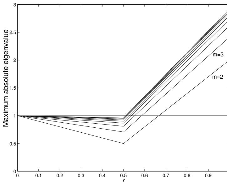
Figure 36.1: Maximum absolute eigenvalue as a function of  $r$  for the matrix  $A$  from the explicit method for the heat equation calculated for matrices  $A$  of sizes  $m = 2 \dots 10$ . Whenever the maximum absolute eigenvalue is greater than 1 the method is unstable, i.e. errors grow exponentially with each step. When using the explicit method  $r < 1/2$  is a safe choice.
