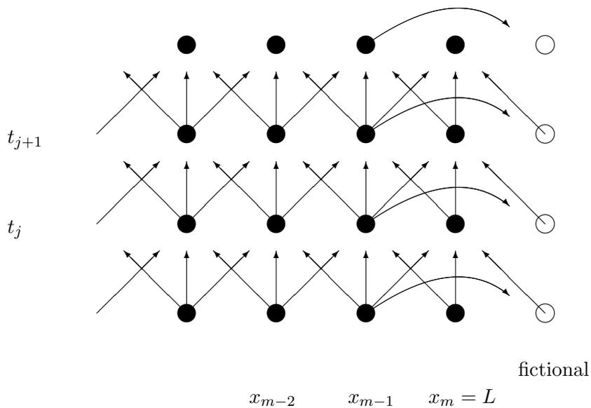
Figure 38.2: Illustration of information flow for the explicit method near the right boundary at  $x = L$ . The top figure shows a fixed boundary condition, where  $u_{m,j}$  is set to be  $g_2(t_j)$ . The bottom figure shows an insulating boundary condition. Now  $u_{m,j}$  is updated in the same way as the general  $u_{i,j}$  and an additional entry  $u_{m+1,j}$  is used with its value set by copying  $u_{m-1,j}$ .
