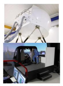
Figure 7.10 AW109 LUH Flight Simulation Training Device (full motion and fix based)
