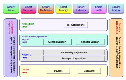
Figure 3.4 IoT Layered Architecture (Source: ITU-T)
