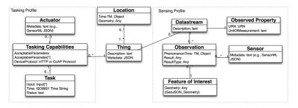
Figure 4.3 SensorThings IoT Resources Model
