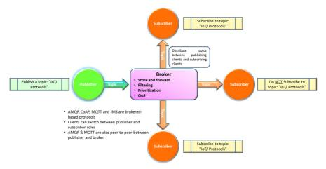
Figure 3.50 Broker based architecture for data exchange protocols
