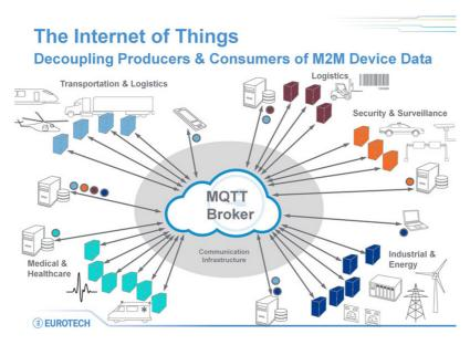
**Figure 3.49** Message Queuing Telemetry Transport publish/subscribe protocol used to implement IoT and M2M applications (Source: Eurotech)
