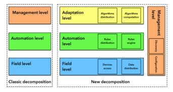
Figure 3.33 Level based architecture of building automation systems [48]
