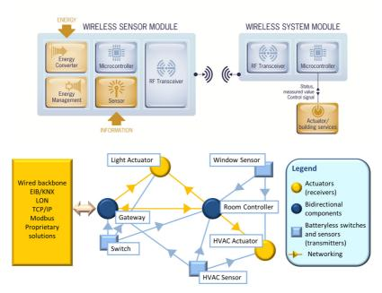
Figure 3.47 Energy harvesting wireless sensor network (Source: EnOcean)
