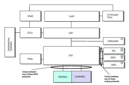
Figure 8.7 Software architecture for Smart Parking
