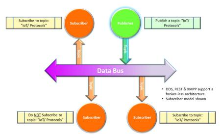
Figure 3.51 Bus-based architecture for data exchange protocols
