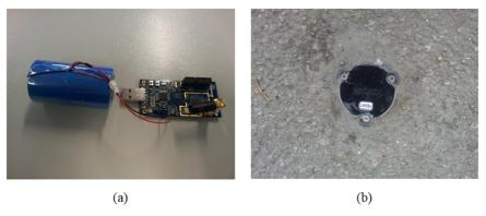
Figure 8.8 Tmote with battery ready for boxing, and (b) Tmote in the Worldsensing box in the real deployment
