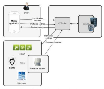
Figure 6.3 Smart Office IoT Context View Diagram
