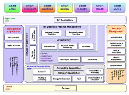
Figure 3.5 Detailed IoT Layered Architecture (Source: IERC)
