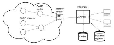
Figure 8.6 Scheme of the implemented HTTP/CoAP caching system
