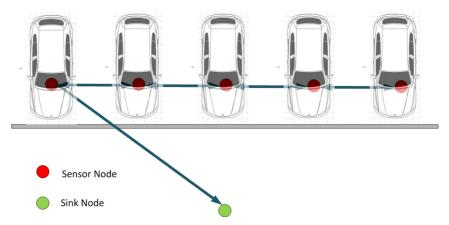
Figure 8.10 Configuration of the network topology
